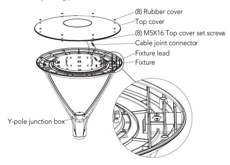
4. (1) Unscrew the waterproof plug pull the fixture lead, center luminaire on tenon and tighten supplied set screws to securely mount luminaire to tenon and pull the fixture lead.
