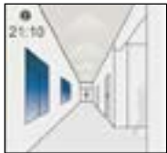
With insufficient natural light, the sensor switches on the light automatically when presence is detected.
