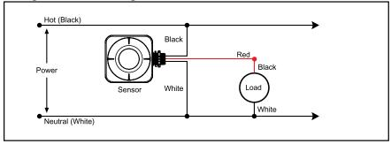
Wiring with dimming ballast or LED driver
