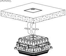
2. Loosen the 2pcs M4 screws (Which is only secured the back housing) and fix the back housing to the ceiling using mounting screws (provided by others).
