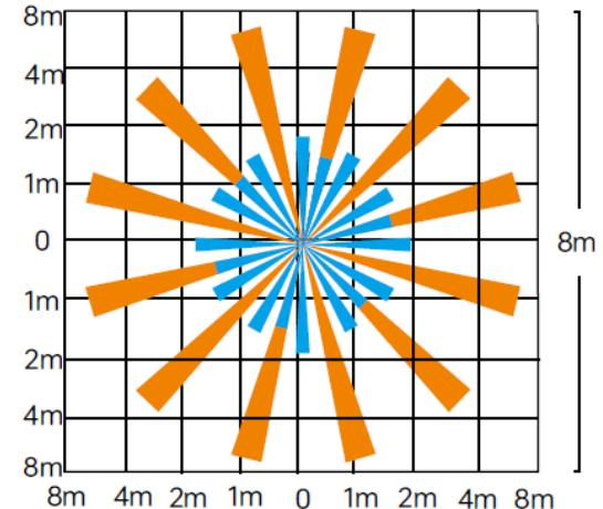
The detection area for movement sensor can be roughly divided into two parts:
