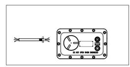
3. Remove the junction box cover (spiral cover) and insert the power cable into the junction box. Then connect the AC cable: black cable joins to L, white cable joins to N, green cable joins to grounding. Further, fill 16mm of chemical filler into the conduit and fix the conduit to the lamp body (it must be confirmed whether there are suitable gaskets before installation).
