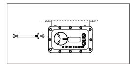
3. Remove the junction box cover (spiral cover) and insert the power cable into the junction box. Then connect the AC cable: black cable joins to L, white cable joins to N, green cable joins to grounding. Further, fill 16mm of chemical filler into the conduit and fix the conduit to the lamp body (it must be confirmed whether there are suitable gaskets before installation).
