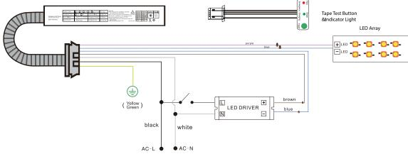
1. IN EMERGENCY MODE, DOUBLE-CLICK THE TEST SWITCH TO TURN OFF THE CURRENT EMERGENCY STATE. 2.TEST ACCESSORY LEADS-OBSERVE PROPER POLARITY WIRING.
