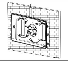
3. Drilling out the holes (C) to secure it on the wall with choosing proper screws.
