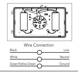
5. Replace the lens on the hinges, make connections and close the lens set then tighten the screws.
