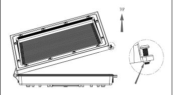
2. Drill appropriate knockouts (B) for wiring, the fixture supports standard 3 1/4" and 4"Junction box.
