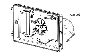
3. Attach the back plate on the wall, use the supplied gaskets for a weather tight seal.
