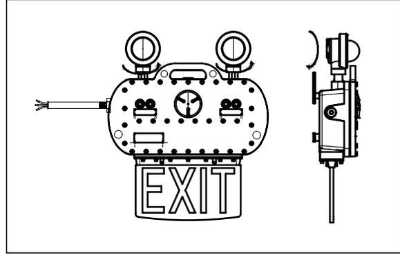
4. After installation, adjust the direction of the headlights as needed.
