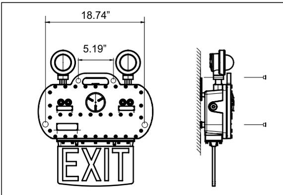
1. Drill four holes as fig. 1, the distance as per 18.74" and 5.19"
