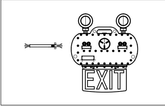
3. Install pipe to 3/4" NPT entry and fix 0.63inch Chico A. Then connect the AC cable: black cable joins to L, white cable joins to N, green cable joins to grounding.
