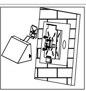
4. After hanging the lamp on the mounting plate and tightening the screws, put a waterproof glue seal between the bottom cover and the wall to prevent water from entering the lamp.
