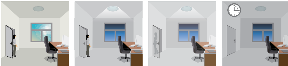
With sufficient natural light, the light does not switch on when presence is detected
