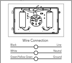
5. Replace the lens on the hinges, make connections and close the lens set then tighten the screws.
