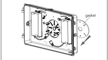
3. Attach the back plate on the wall, use the supplied gaskets for a weather tight seal.
