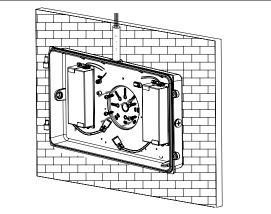
3. Drilling out the holes (C) to secure it on the wall with choosing proper screws.
