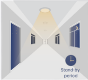
Sensor dims light to standby dimming level after hold time if there is still no motion.
