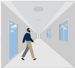
With sufficient daylight, the sensor keeps light OFF even motion gets detected.
