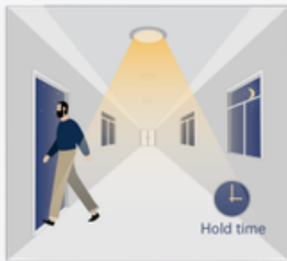
After there's no motion detected, the sensor keeps light ON 100% for hold time.
