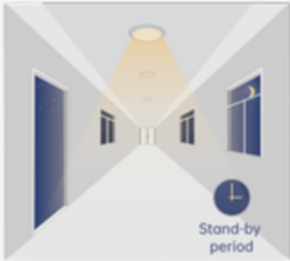
After hold time, sensor dims light to standby dimming level for standby period. If the standby period has been set as 0s, sensor turns light OFF automatically after hold time.
