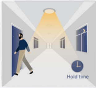
Sensor keeps for a hold time period after motion leaves.
