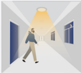
With insufficient daylight, the sensor turns light ON when motion gets detected.
