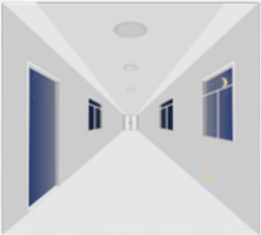
The sensor turns OFF light automatically after the standby period when there's no motion detected.
