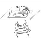
Push clips up & install into fixture
