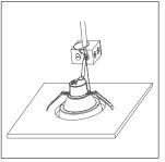
Ensure fixture is flush. Installation is complete
