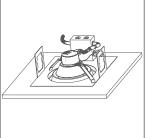
Ensure fixture is flush. Installation is complete
