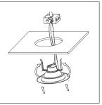
Push clips up & install into fixture
