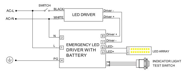
1.DO NOT MATE CONNECTOR UNTIL INSTALLATION IS COMPLETE AND AC POWER IS SUPPLIED.
