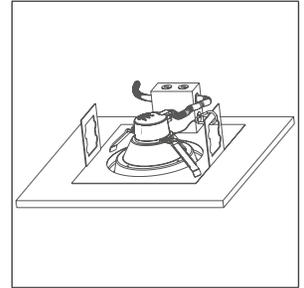
Ensure fixture is flush. Installation is complete
