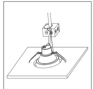
Ensure fixture is flush. Installation is complete
