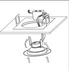
Push clips up & install into fixture
