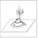
Ensure fixture is flush. Installation is complete
