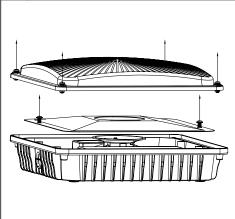
2. Cut off the wires through the 3/4" hole and plug the hole with provided Plug. Drill 4 holes on the edge of the fixture and fix it on the ceiling using the appropriate screws.
