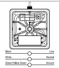
5. Re-attach lens and metal plate, make sure no wires are pinched
