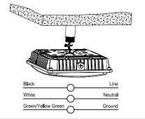
3. Screw the Conduit into the hole on top of the Canopy.
