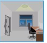
The light dims to stand-by period after hold-time and stays on selected minimum dimming levels.
