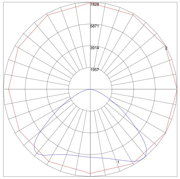
Maximum Candela = 7827.788 Located At Horizontal Angle = 0, Vertical Angle = 37 # 1 - Vertical Plane Through Horizontal Angles (0 - 180) (Through Max. Cd.) # 2 - Horizontal Cone Through Vertical Angle (37) (Through Max. Cd.)
