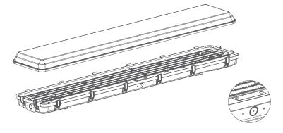
2. Remove the plastic screw and remove the cover.
