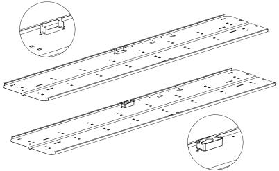
5. Connect the sensor to the driver refer to General Wiring Diagram. Reinstall the LED tray and fixture lens.
