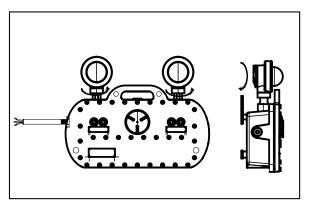
4. After installation, adjust the direction of the headlights as needed.
