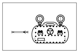
3. Install pipe to 3/4" NPT entry and fix 0.63inch Chico A. Then connect the AC cable: black cable joins to L,white cable joins to N, green cable joins to grounding.
