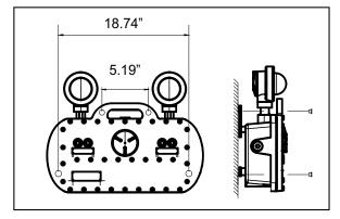
1. Drill four holes as fig. 1, the distance as per 18.74" and 5.19"
