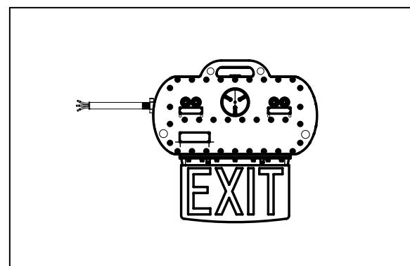
4. Connect the AC cable: black cable joins to L, white cable joins to N, green cable joins to grounding.
