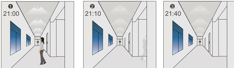
The light switches on at 100% when there is movement detected. The light dims to stand-by levels after the hold time. The light remains in dimming level at night.
