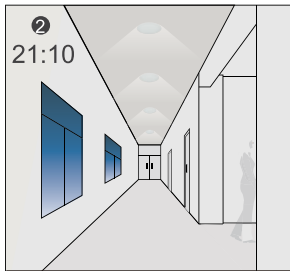
The light dims to stand-by levels after the hold time.
