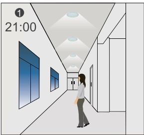
The light switches on at 100% when there is movement detected.
